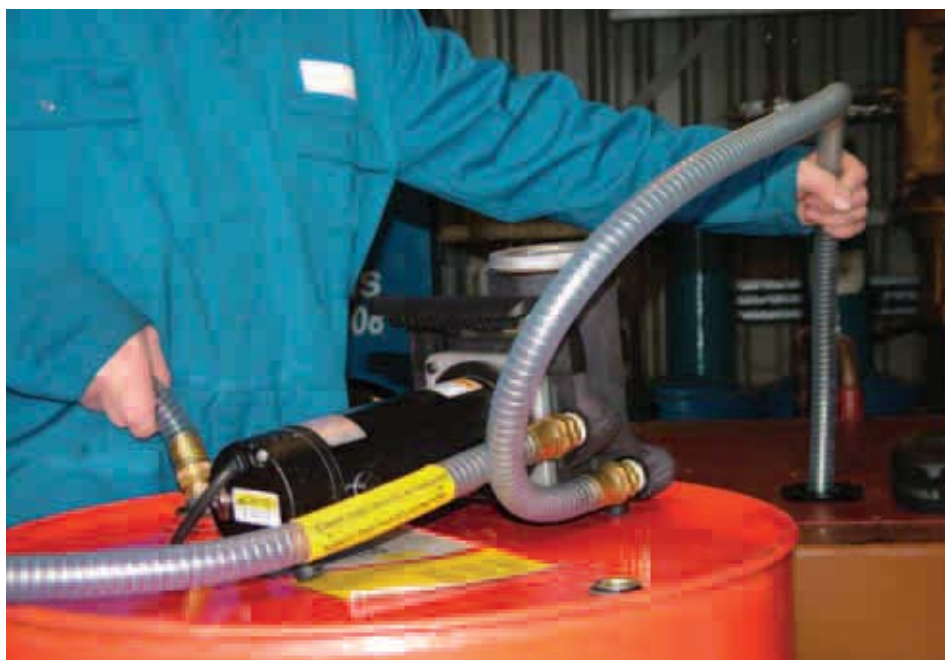
Alternative customer selectable inlet and outlet ports (plugged)
