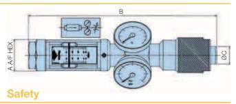
An axial flow restrictor valve is fitted which can be adjusted under full load from open to fully closed, and to complete the specification, a safety blow-out disc, set to fail at 455 bar is fitted to the manifold in a position facing away from the operator when reading the gauges normally. Two spare blow-out discs are supplied which are easily replaced by removing the hexagonal plug on the gauge manifold.
