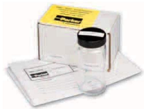
**ParTest™** fluid analysis. For complete analysis, Parker offers Par-Test fluid analysis. Your Parker representative can supply you with a fluid container, mailing carton and appropriate forms to identify your fluid and its use. An independent lab performs complete spectrometric analysis, particle counts, viscosity and water content.
