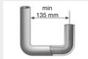
● Minimum clearance of U-shape bends
