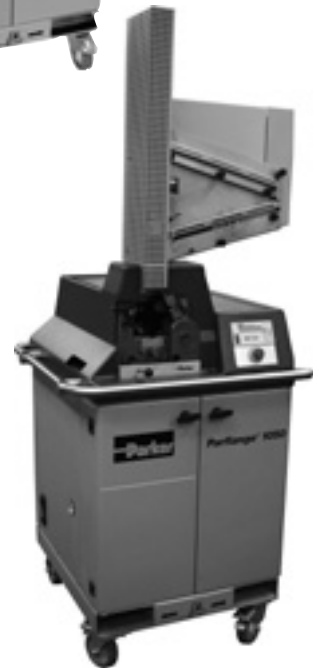
Parflange® 1050 PRO for mass production of O-Lok® assemblies
