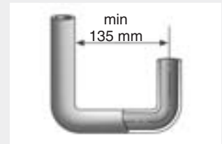
● Minimum clearance of U-shape bends
