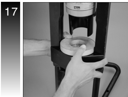
Place silver die ring on top of die. Position ring so it is centered on die.
