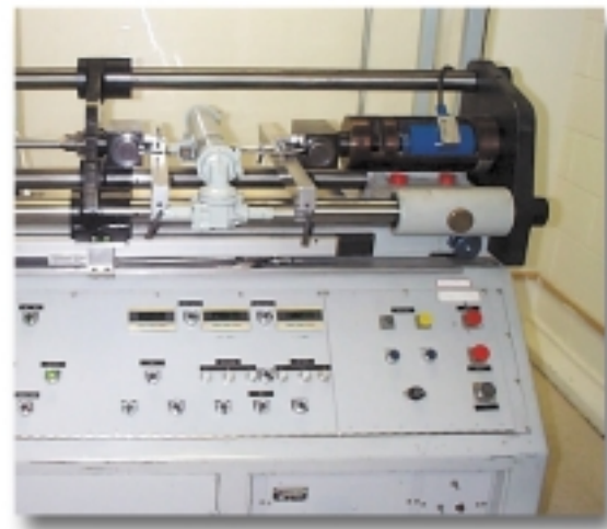
This linear actuator test bench is part of an automated test system. Benches can be built to accommodate a wide variety of actuator size and force. Shown here with a small linear actuator under test, this bench can burn-in and test many actuator types.
