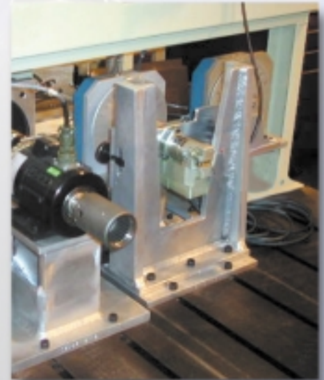
This rotary actuator test bench allows flexible mounting of many sizes and types of actuators. Quick change mounting and coupling adapters can be provided by Testek for several test components, or for your entire fleet.
