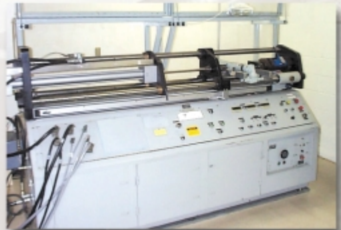
Linear actuator test benches can be built to accommodate multiple large and small components. This bench is part of a computer aided test installation for defense aircraft support.
