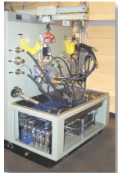
This is the front of a fuel pump/fuel boost pump test stand. This test stand features a separate operator console located outside the test cell. The test stand is shown with most access and maintenance covers removed. Note hoists to aid operator in placing the test part on the drive pad.
