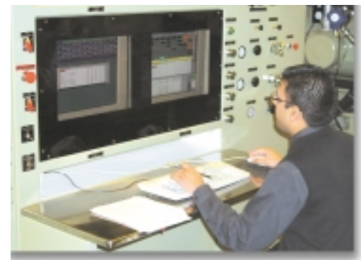
This remote operator console provides a safe and comfortable station for test operators. The two color displays show all test parameters, as well as the test program, test report (as it is being written), and graphical displays of schematics and hookup diagrams for each unit. TestEx runs on PC computers with the latest Windows operating system. Operators quickly become familiar with the use of standard keyboard and mouse controls, and rely on TestEx for safety and protection of the test part and test stand.
