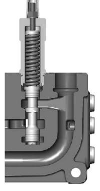
PLS - limiting function which maximise the differential pressure between the pump pressure and the load signal.
