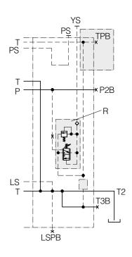
R [37] internal pilot-pressure supply. YS [39] adapter for connection of external pilot-pressure filter.
