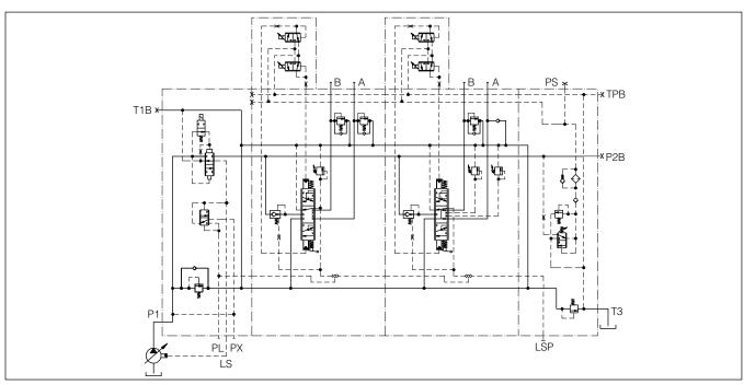
Principle circuit diagram for valve with load sensing.
