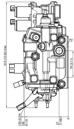
With MU section, the L dimension is reduced by 23 mm (0.91) With IP section, the L dimension is reduced by 25 mm (0.98) For connection thread, please refer to page 7.
