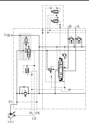
BEN - Electrically controlled pump-unloading function.
