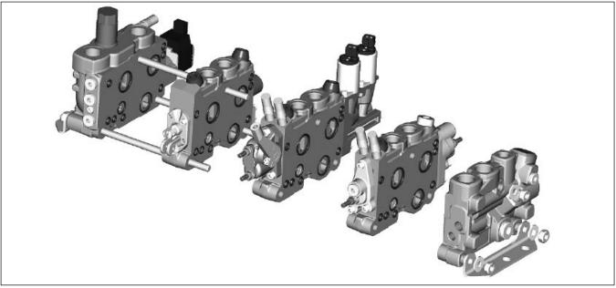
The L90LS is a stackable, multi-section, load-sensing, pressure-compensated directional valve for mobile machines such as cranes, skylifts, forklift trucks, platform trucks, excavators and harvesters. It is designed for working pressures of up to 320 bar and a maximum pump flow of 200 l/min. The valve can be given excellent simultaneous-operating characteristics, which enable several machine functions to be operated responsively at the same time, regardless of the sizes of individual loads.
