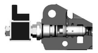
BEN - Electrically controlled pump-unloading function.
