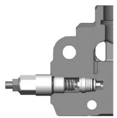
PLM – Pressure relief valve for inlet section AS and AS2.
