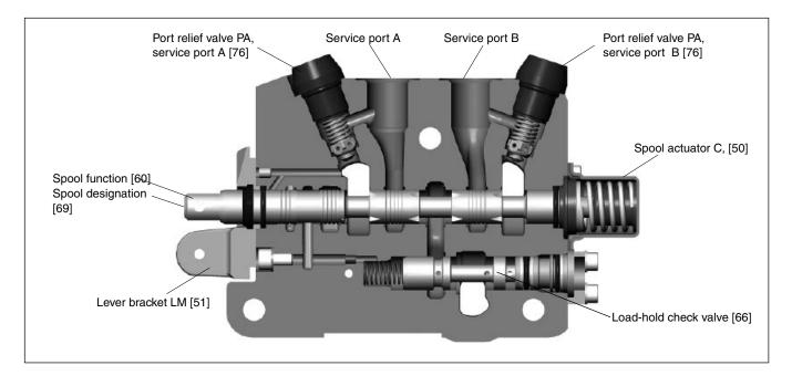
Spool actuators of both the open and enclosed type can be used on the L90LS. Open spool-actuators, in which the spool-end is exposed, are simpler and cheaper. They are intended for use in systems where low capital cost is a priority. They can be operated directly by means of linear levers or can be connected to remote controls by means of wires.
