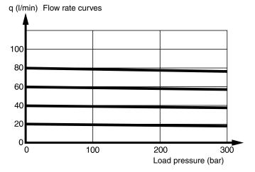
Load-independent flow with pressure compensator.
