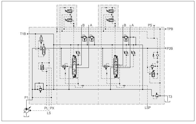
L90LS with electro-hydraulic remote-controlled spool actuators and equipped with direct-acting main pressure relief valve for systems fed by LS pumps, pump-unloading function, integrated pilot-oil supply, counter pressure function, section-specific pressure compensators, port-specific feed reducing valves, port-relief and anti-cavitation valves, etc.
