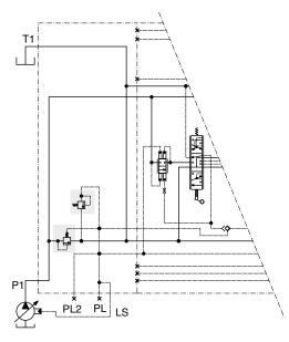
AS – Inlet section for flow-sharing valve.
