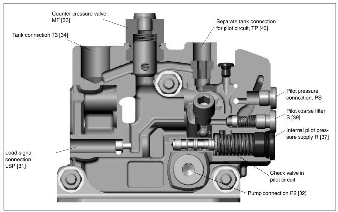
US End Section with pilot pressure supply, pilot filter, Counter pressure valve and separate tank connection for pilot circuit.
